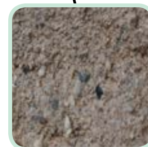
Lime based mortar with big ceramic, tuf and sand particles
