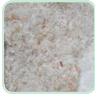
Hydraulic lime with sandstone particles
