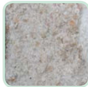
Hydraulic lime with sandstone particles
